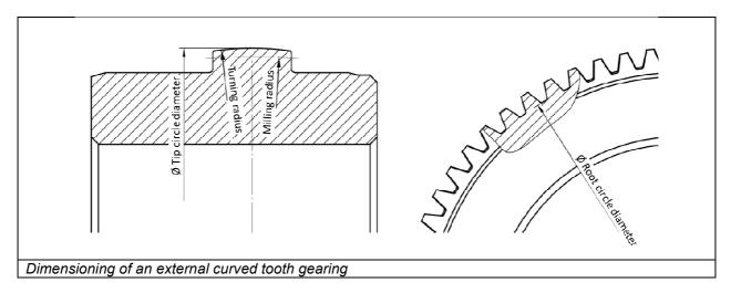
The production drawing of the internal gearing requires the root circle diameter and the tip circle diameter in addition to the gearing mark.
